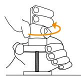
To remove, hold base of Scotty Mount firmly and twist barrel until connector thread is fully extended
