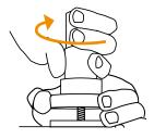
Hold base of the Scotty Mount firmly and turn barrel clockwise
